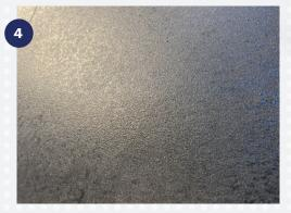
After complete drying the **film should be homogeneous** and not sticky.
